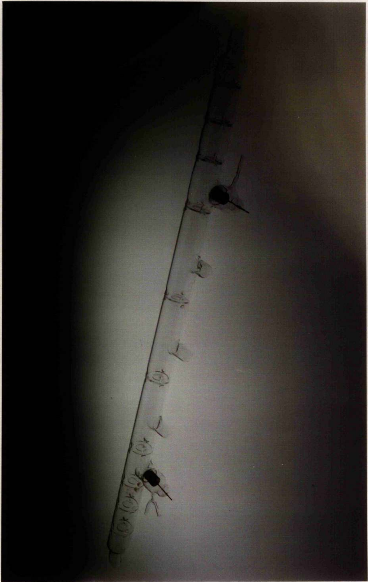
Figure 6.7. Second sidearm laser tube showing diaphragms and electrodes.
