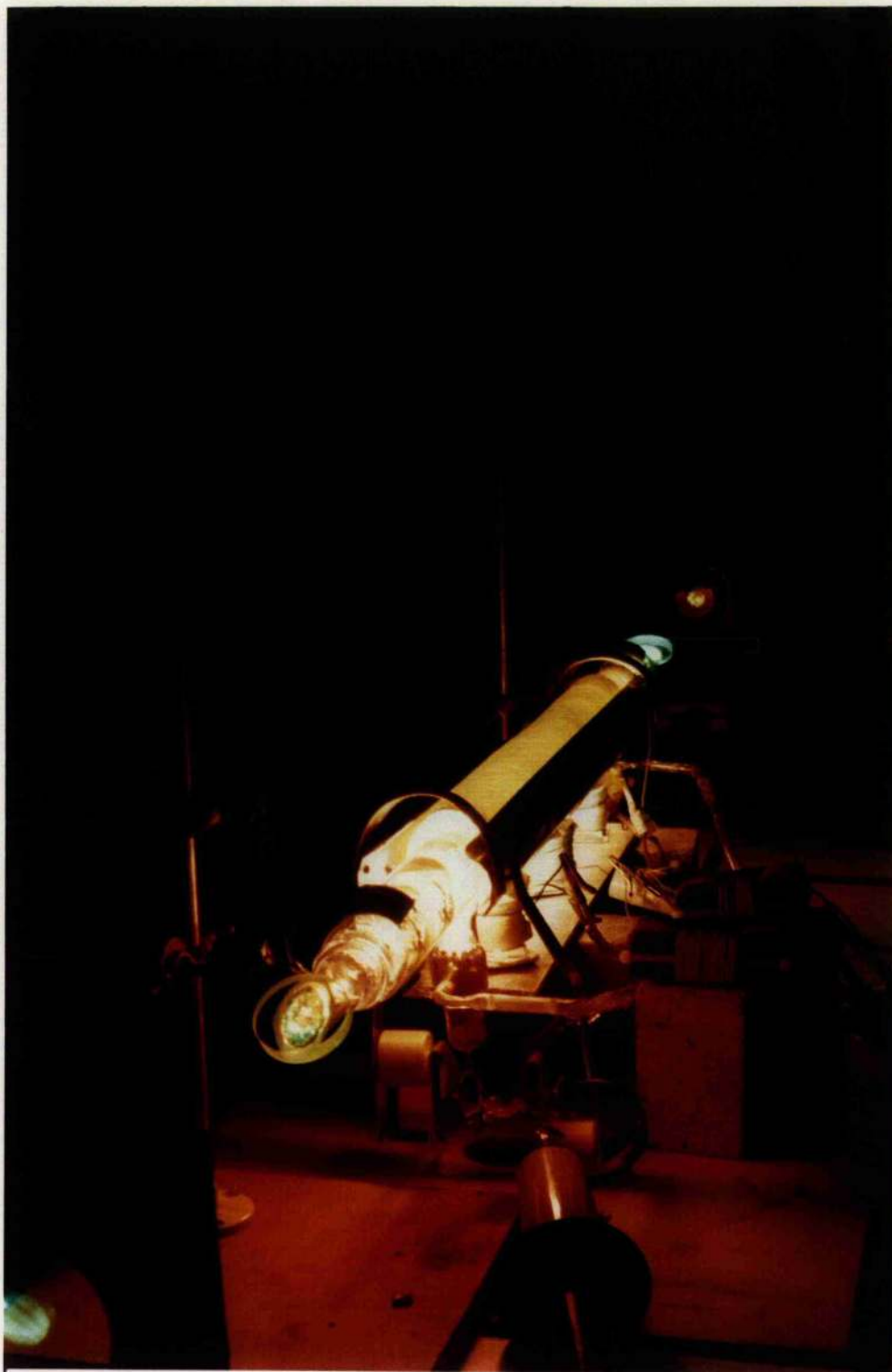
Figure 6.8 Sealed-off sidearm tube in operation.
