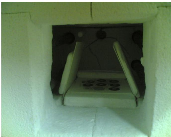
Figure 3.7 Setup inside furnace chamber for sintering BCZYZnO green tapes.
