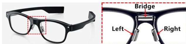
Figure 1 J!ns Meme and its EOG electrode placement.
