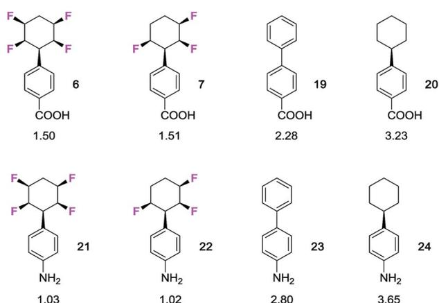
Fig. 3 Measured<sup>20</sup> log *P* values for benzoic acid and aniline derivatives of selectively fluorinated cyclohexanes.
