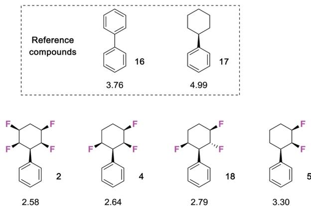
Fig. 2 Measured<sup>20</sup> log *P* values for compounds selectively fluorinated phenylcyclohexanes and reference compounds 16 and 17. Increasing fluorination lowers log *P* consistent with increasing hydrophilicity.
