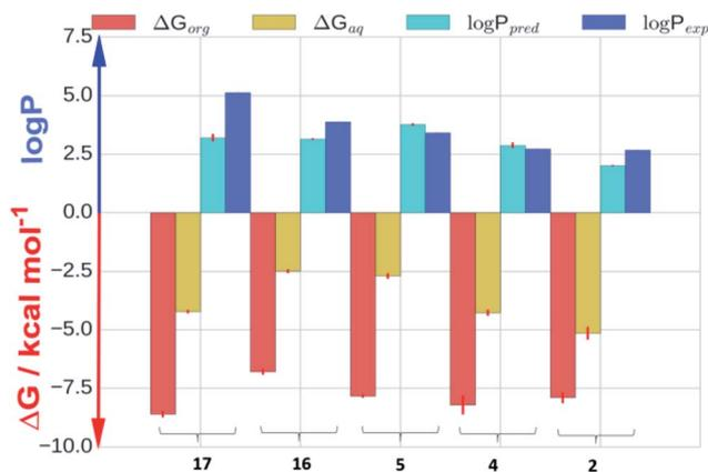
Fig. 4 The positive y-axis depicts a comparison between calculated (cyan) and measured (blue)  $\log P$  values for compounds 2, 4, 5, 16 and 17. The negative y-axis depicts calculated solvation free energy in cyclohexane,  $\Delta G_{org}$  (red), and aqueous,  $\Delta G_{aq}$  (yellow), phases.
