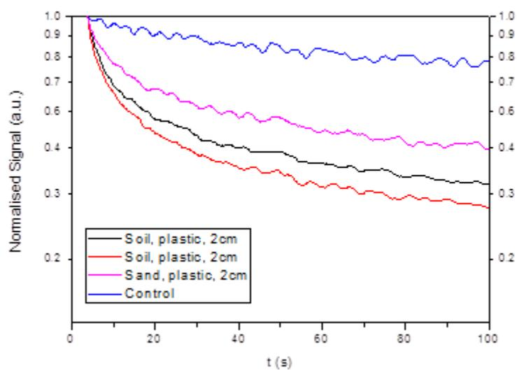
Fig. 8. Comparison of Super Yellow films with 2,4-DNT (black and red lines) and TNT (green line) against blank (blue line), with the explosives buried at 2cm under soil in plastic.
