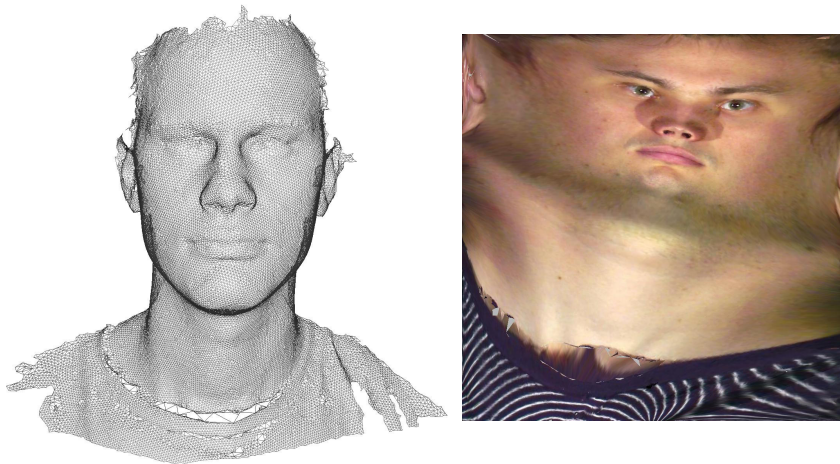
Figure 5.1.1.: The 3D camera provides separate files for shape (left, surface depth map) and textural information (right).
