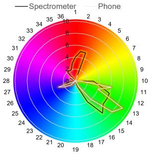
Figure 6. Results for color detection, the black and white line show where error occurs for the spectrometer and the phone, respectively. The inner numbers are the number of errors (out of 10) and the outer numbers are the hue angle (divided by 10). We can observe that the errors occur near to the three dominant colors, especially for green color.
