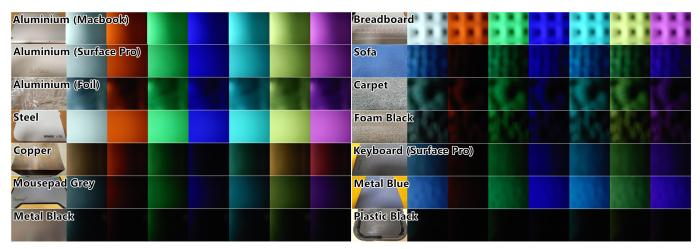
Figure 3. Sample materials and the captured images with the reflected colors on (left) metallic materials and (right) textured materials.
