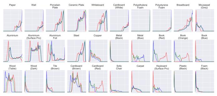
Figure 4. Color histogram of visually similar materials: (top) white and grey (middle) metal and books (bottom) brown, dark and textured materials. The x-axis represents the 64 color bins whereas the y-axis represents the amplitude and is automatically scaled for clarity, which can be seen in the varying grid. Note that this is the color histogram of the white image only. Using more features from other color can improve the accuracy further.
