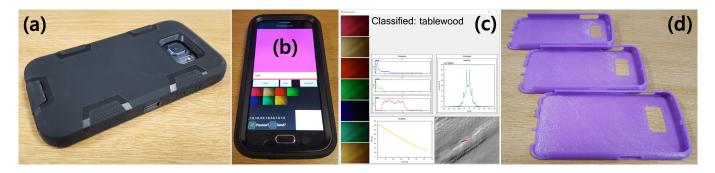
Figure 1. a) The phone is facing down while the screen flashes different colors and the camera captures images of the reflected light. b) The UI of the phone, showing the main light source and the captured images. c) The UI of the classification server, showing the received images, the classification results on top and the extracted features (color histogram, gradient, etc). d) 3D printed cases with different height for the pilot study.
