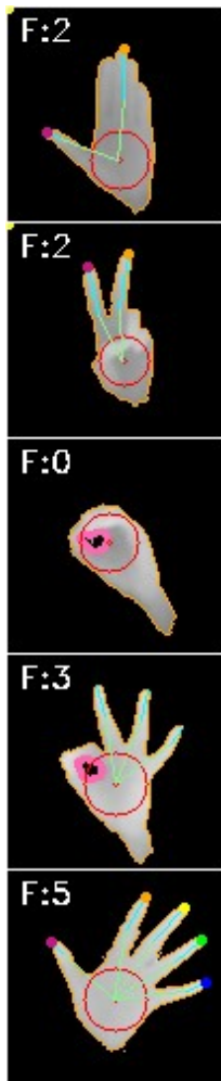
Figure 3: Different static gestures can be recognized, top to bottom: L, lasso, O, OK, rotation.
