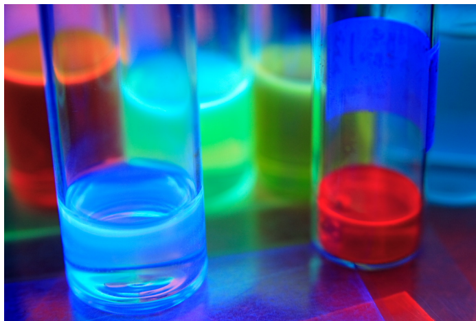
Figure 2.6 Various organic semiconductors emitting across the visible spectrum under UV illumination.
