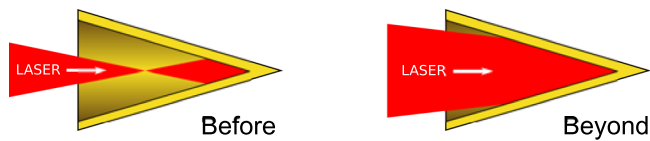
FIG. 1. Focusing the laser before the cone tip and beyond the cone tip.
