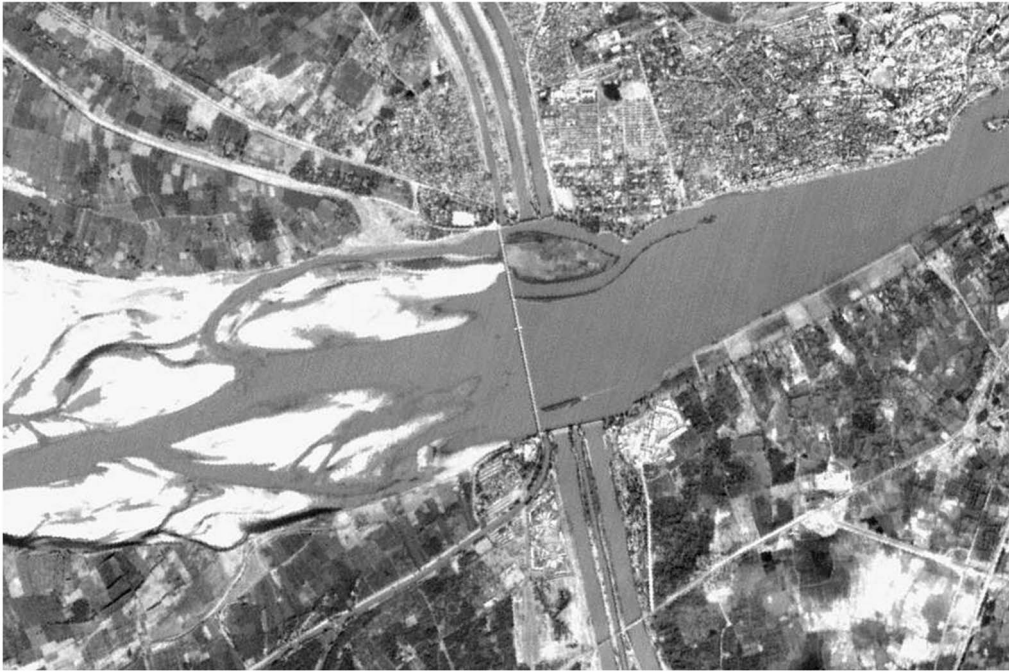
Figure 2. Aerial photograph of Sukkur Barrage. Image shows the seven canals diverting water out of the river, and demonstrates the dramatically reduced flows downstream (river flow direction right to left). doi:10.1371/journal.pone.0101657.g002
