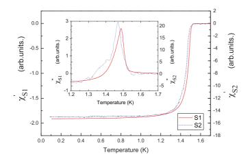
FIG. 1. (Color online) Real part of ac susceptibility data measured through the critical temperature of the two crystals studied here. The inset shows the imaginary part of the ac susceptibility near  $T_c$ .
