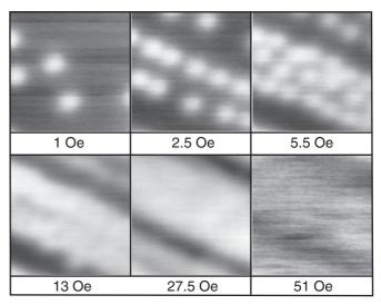
FIG. 7. SHPM images captured parallel to the *a-b* face of the same region of sample 2 after field cooling from above  $T_c$  in the indicated applied fields ( $H \parallel c$  axis). Vortices are white; scan size  $\approx 14 \times 14 \ \mu$ m;  $T = 330 \ m$ K. Grayscale ( $\Delta B$ ) spans 1.98, 2.13, 1.89, 2.7, 2.55, and 0.89 G, respectively.
