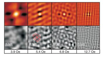
FIG. 3. (Color online) SHPM images captured parallel to the *a-b* face of sample 1 after field cooling from above  $T_c$  in the indicated applied fields ( $H \parallel c$  axis). Scan size  $\approx 14 \times 14 \mu$ m; T = 330 mK. The top row shows self-correlation plots of the raw images in the bottom row (vortices are white).
