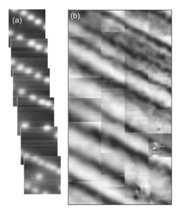
FIG. 5. Composite SHPM images captured parallel to the *a-b* face of sample 2 after field cooling from above  $T_c$  in applied fields  $(H \parallel c \text{ axis})$  (a) H = 2.4 Oe ( $\approx 20 \times 70 \ \mu\text{m}$ ) and (b) H = 15.7 Oe ( $\approx 45 \times 70 \ \mu\text{m}$ ). T = 330 mK.
