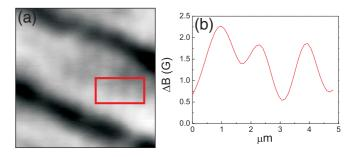
FIG. 6. (Color online) (a) SHPM image captured parallel to the *a-b* face of sample 2 after field cooling from above  $T_c$  in H = 16 Oe  $(H \parallel c \text{ axis})$ . Scan size  $\approx 14 \times 14 \ \mu\text{m}$ ;  $T = 330 \ \text{mK}$ . (b) Average of the *x*-scan lines in the region indicated in (a) showing the presence of vortex chains within the bands.
