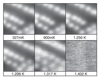
FIG. 9. Temperature dependence of SHPM images captured parallel to the *a-b* face of the same region of sample 2 after field cooling from above  $T_c$  in H = 2.4 Oe ( $H \parallel c$  axis). Scan size  $\approx 14 \times 14 \mu m$ .
