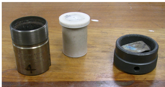
Figure 2.1: Steel autoclave ( left ) and screw top ( right ) with a PTFE liner ( centre ).
