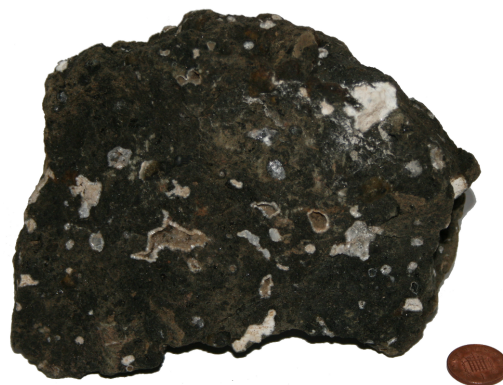
Figure 1.4: Photograph of vesicular lava (Staffin, Skye, UK). Vesicles, formed by gas within the lava, are filled with zeolite (white crystals) crystallised from \text{Al}^{3+} or \text{Si}^{4+} fluids which flowed through the lava after cooling. One penny coin for scale.
