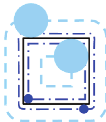
Figure 2.10: The effect of edges and corners on the accessible surface area. After Düren et al.[173]
