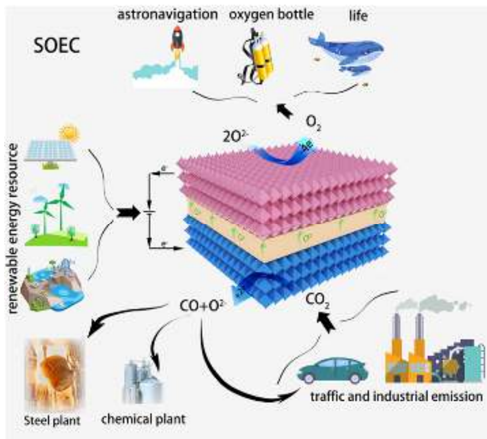
Figure 1. Schematic diagram of energy conversion and storage based on solid oxide electrolysis cells technology.
