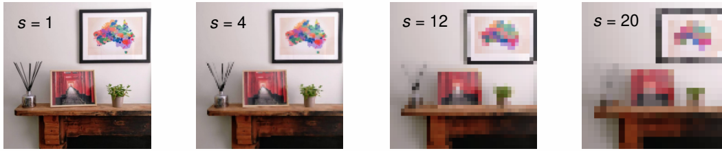
Figure 2: Effect of sub-block size, s . No pixelation is s = 1 up to a maximum value of s = 20 (pixelation at 20 \times 20 pixels).
