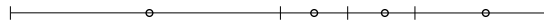
Fig. 1. The 1D grid with centres \{\frac{1}{4}, \frac{9}{16}, \frac{11}{16}, \frac{7}{8}\} and sizes \{\frac{1}{2}, \frac{1}{8}, \frac{1}{8}, \frac{1}{4}\} is equivalently given by the set \{2, 12, 13, 7\} including the corresponding lines of the matrix C .
