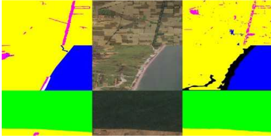
Figure 5.10: Remote Sensing Image Classification. Left: the result from baseline approach provided by [33]. Middle: the corresponding original image. Right: the proposed classification result. Different colors are applied to identify different region classes as used in [33].
