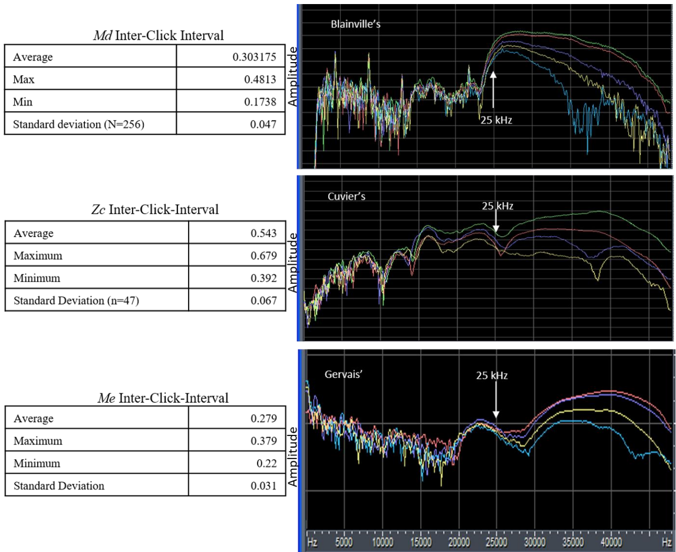
Figure 1.4 Frequency (Hz) vs. amplitude (dB) for successive clicks from an animal's beam moving across a hydrophone for Blainville's (top), Cuvier's (middle), and Gervais' (bottom) beaked whales recorded on the AUTECH Range. Each colour represents a separate click in a click train from highest (top) to lowest (bottom) amplitude.
