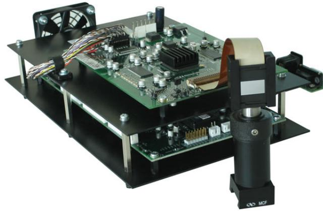
**Figure 3.6:** Image of the Holoeye HEO 1080 P SLM used for these experiments. Image from the Holoeye website [143].
