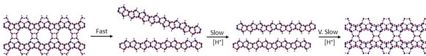
Fig. 1. A schematic representation of the ADOR process from parent germanosilicate UTL . Step 1 proceeds through the fast hydrolysis in water to form the disordered IPC-1P layers. Upon treatment with hydrochloric acid these layers begin to rearrange themselves (step 2). Finally, in step 3, the rearrangement is coming to an end and the new daughter zeolite is beginning to be formed. Upon calcination IPC-2 (shown here) would be afforded. The rate of the final two steps are greatly increased by an increase in molarity of acid, [H^+] .
