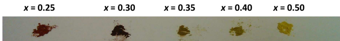
Figure 1: Change in colour of (\text{CH}_3\text{NH}_3)_{1-2x}(\text{H}_3\text{NC}_2\text{H}_4\text{NH}_3)_x\text{PbI}_3 with increasing ethylenediammonium content.
