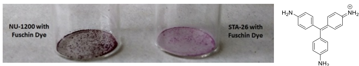
Figure 15. NU-1200 and STA-26(Zr) after exposure to a solution of Fuchsin basic dye (right).
