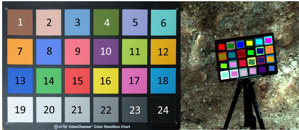
Fig 2 Left: Image ROIs must be created in the order shown above in order to be correctly read into ExoSpec. Right: An example of ROIs selected and overlaid on the calibration target in an LWAC scene.
