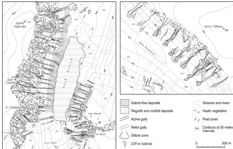
Figure 18 Debris flows and debris cones on the flanks of glacial troughs: Gleann Einich, Cairngorms (left) and Glen Docherty near Kinlochewe (right). Adapted from a map in Curry (1999a) and reproduced with the author's permission.
