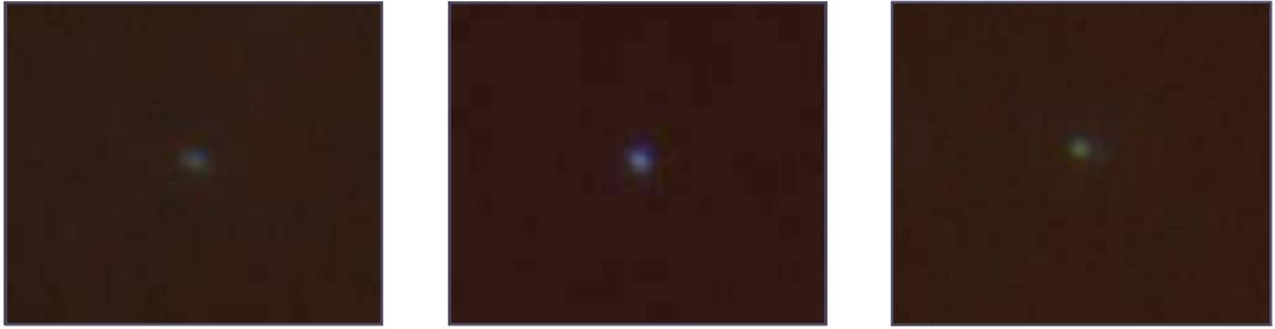
**Figure 3.14:** Silver nanoparticles held in a single beam trap with 40nm, 60nm and 80nm diameter (from left to right). The scattered light from the nanoparticle increases with size. The colour of the silver nanoparticles changes from blue to green due to the redshifting of the resonance for larger particle sizes.
