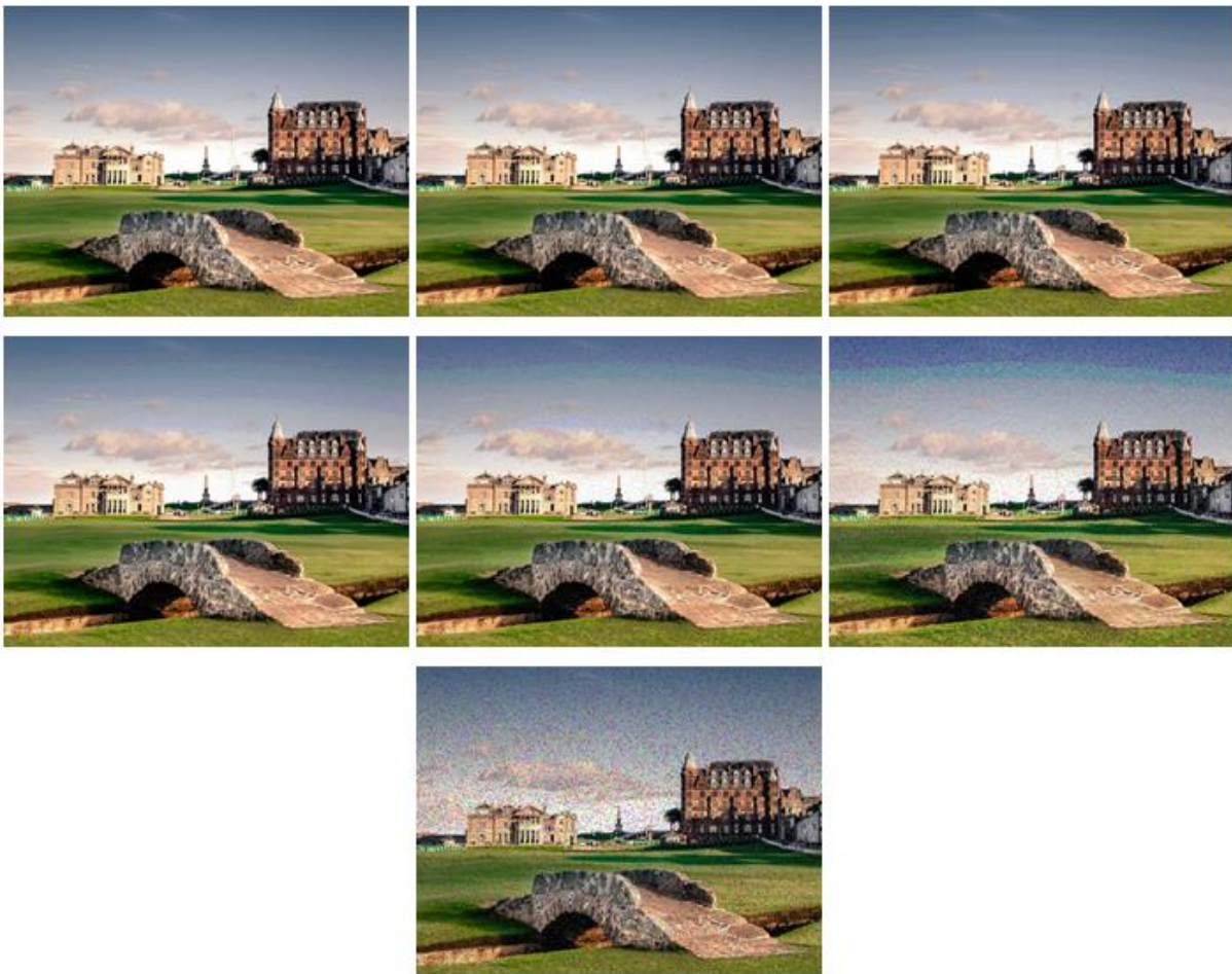
Figure B28: Stego images from LSB 2 to LSB 8, with a large size data file. LSB 1 is not enough to conceal the secret data file.
