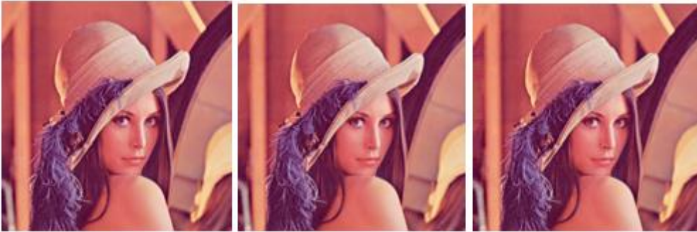
Figure 70: The stego image results in LSB 1, LSB 3 and LSB 5, in Lena.bmp, with a small size data file.
