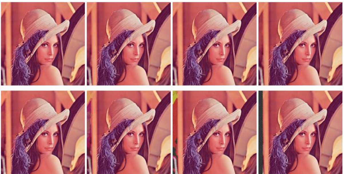
Figure B14: Stego images from LSB 1 to LSB 8, with a small size data file.
