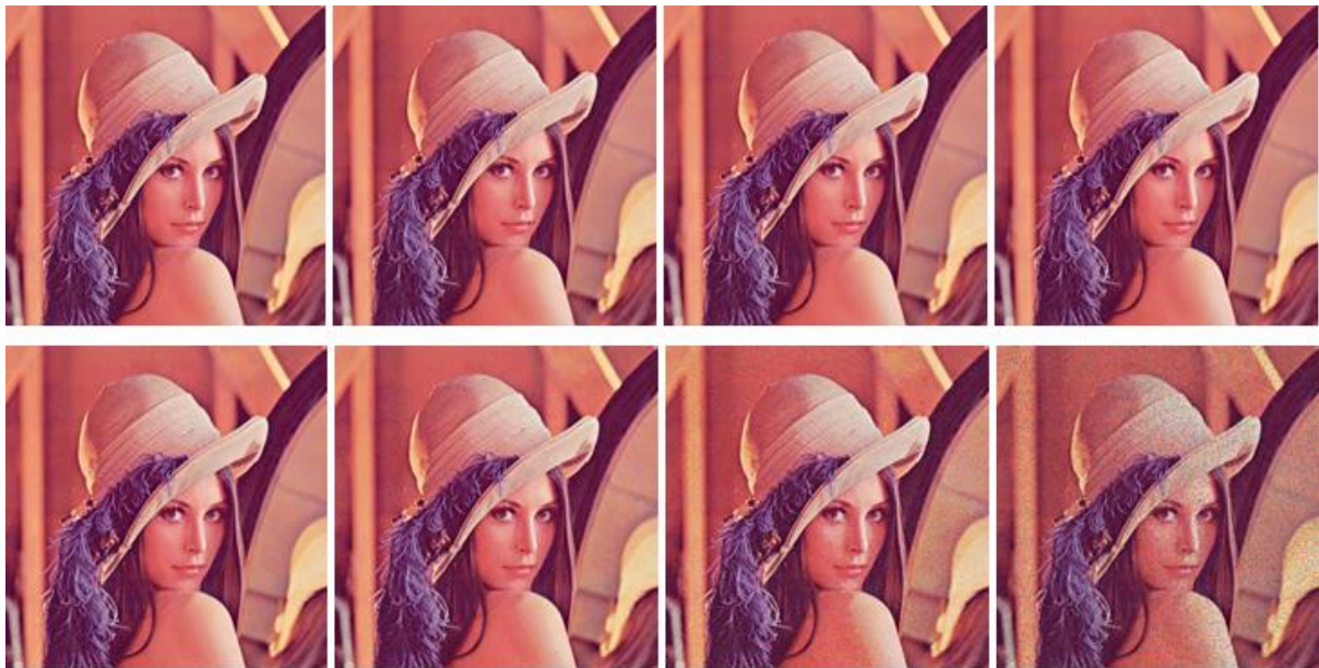
Figure B25: Stego images from LSB 1 to LSB 8, with a large size data file.
