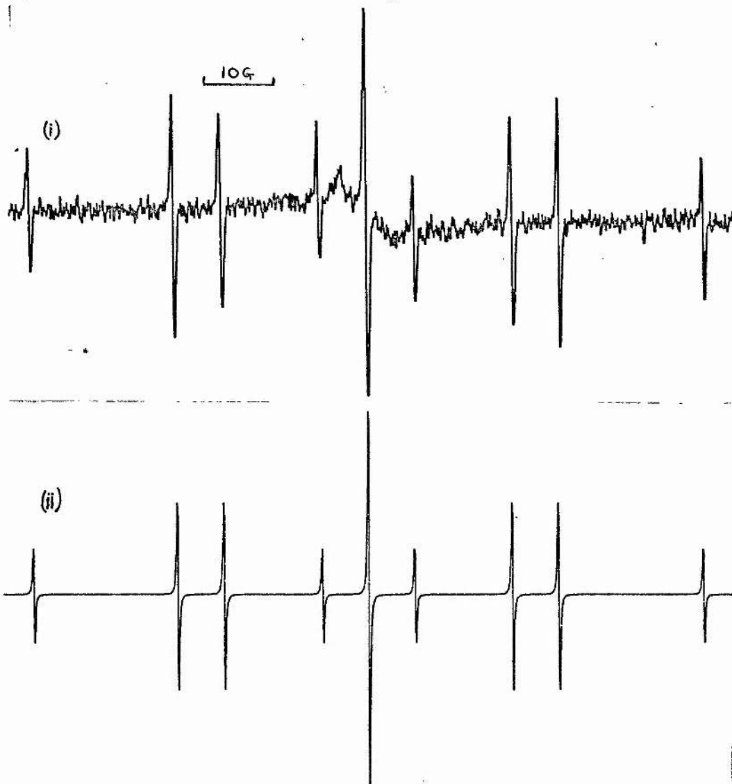
Figure 8. Whole spectrum of cyclobutenylethyl radical (17b) at ca 9.4GHz, 200G scan. (i) observed at 176K, (ii) simulation
