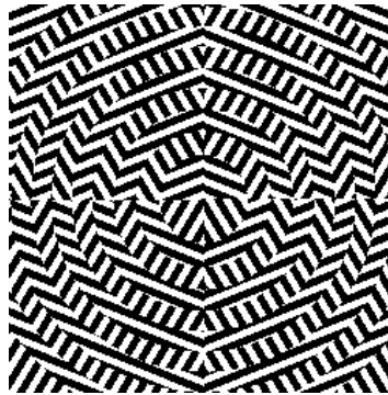
Fig. 3. The layout of the grooves of a transmission binary metalens that is capable of simultaneously converting the linear polarization into the radial one and generating a tight focal spot.
