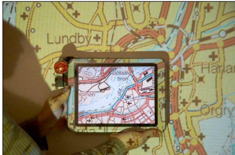
Figure 3.7: Visual Field Contiguous & Depth Non-contiguous: In Ubiquitous Graphics, a user holds up a tablet PC in front of a large projected image to view details (used with permission from [207]).
