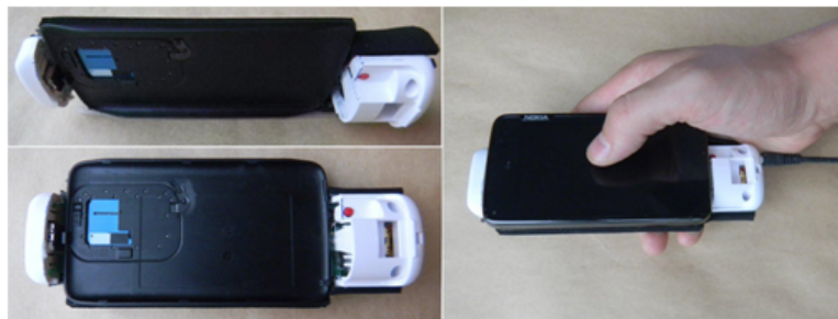
Figure 4.2: Mobile device: Wiimote circuit board attached to the back cover of N900 mobile phone.
