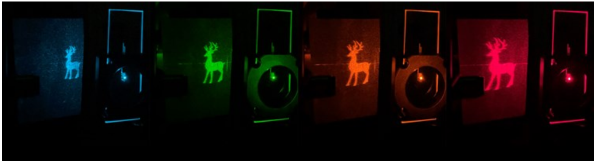
Fig. 6.13. Experimental measurements of the \text{ZrO}_2 HMSs for holographic imaging applications across the visible range.
