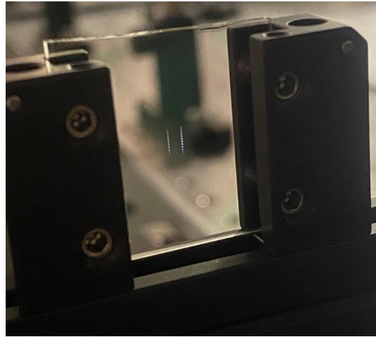
Fig. 3.10. An image showing the MSs on a roughly 7.5 \times 7.5 \text{ cm}^2 glass microscope mounted on a 2D stage for an experiment.
