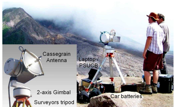
Fig. 1. AVTIS 94-GHz radar/radiometric instrument set up for use in the field on Montserrat, West Indies. The lava dome being scanned is obscured by the volcanic gas plume and lies behind the foreground ridge.
